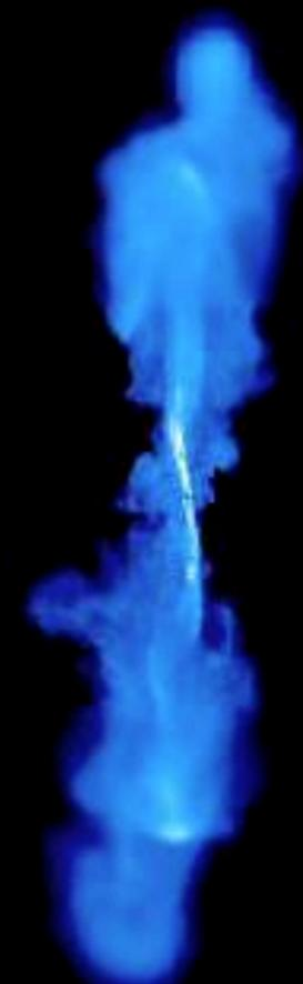
buoyancy velocity > jet expansion velocity
