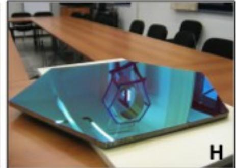
First M1 segments (COR3, most aspheric one) successfully realized in August/September 2012!!
