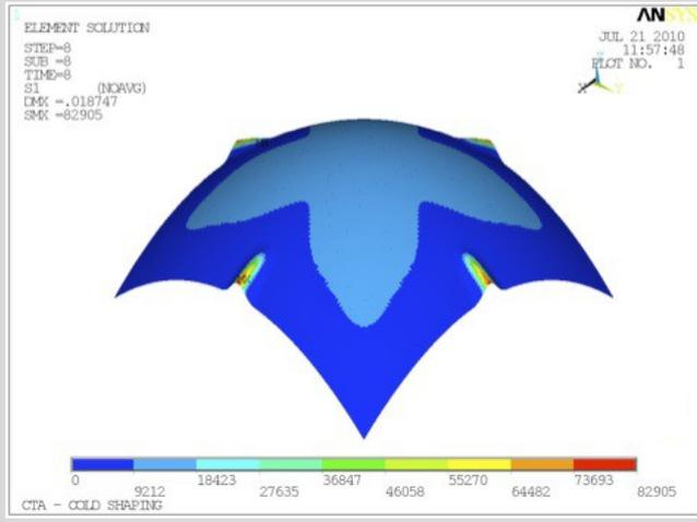
It is made easier by: reducing the curvature; reducing the thickness; increasing the size; changing the geometry from hex to square
