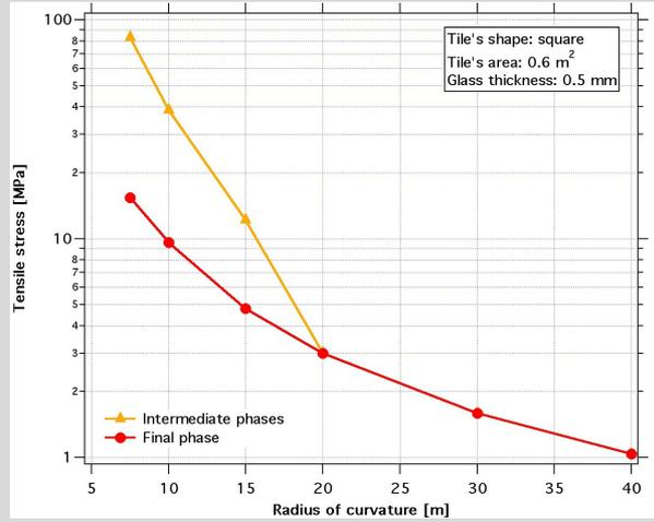
Corrugated configuration: folds not in contact with the mold. At folds location very high stress.
