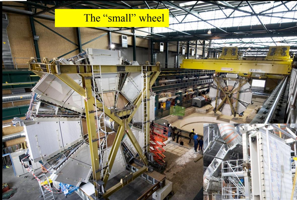
The small wheel have been downloaded after integration of all the muon chambers .
