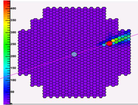
Geometrical determination of the shower impact point on the ground provides a better understanding of the shower geometry.
