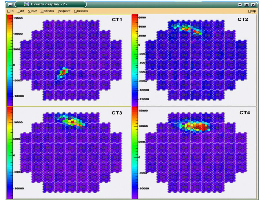
With several telescopes, a stereoscopic (or multiscopic) view of a single shower is possible. This allows to reconstruct the shower geometry and to reject background signals.
