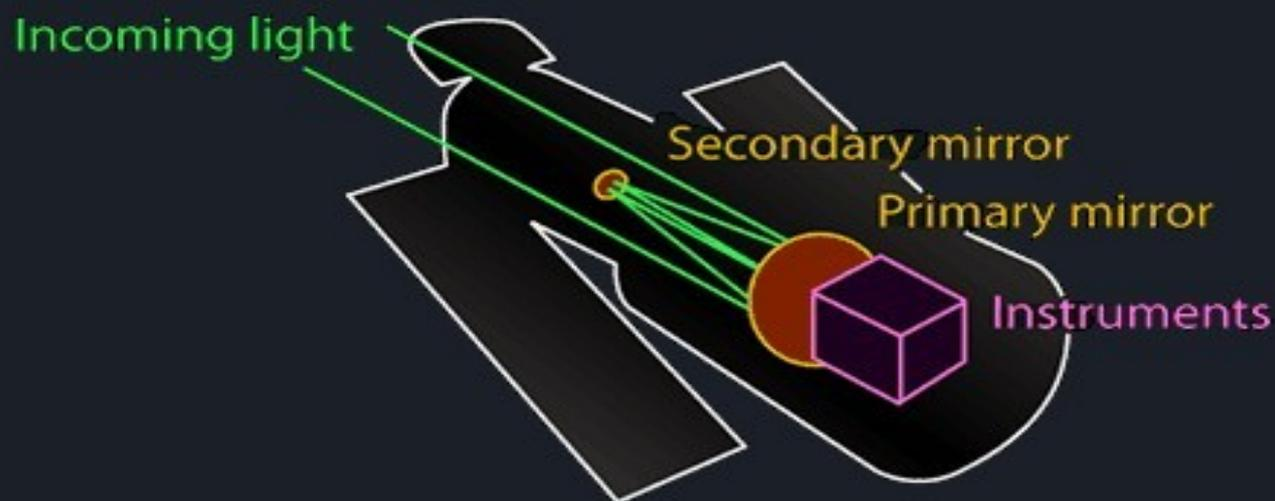
When light strikes the concave primary mirror of the Hubble Space Telescope, it is reflected to the convex secondary mirror, then back through a hole in the center of the primary mirror. There, the light comes to the focal point and passes to one of Hubble's instruments. Telescopes of this design are called Cassegrain telescopes, after the person who designed the first one.
