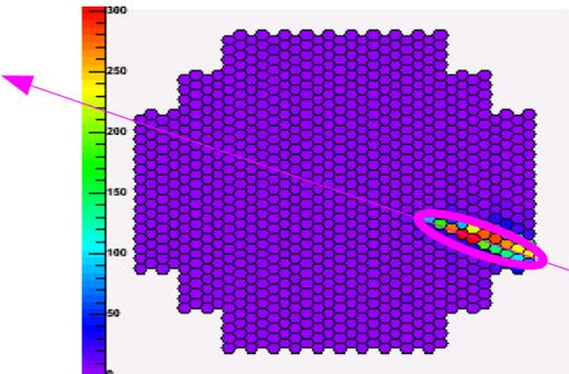
In this case, the air shower came directly from the direction the telescopes are pointing at.
