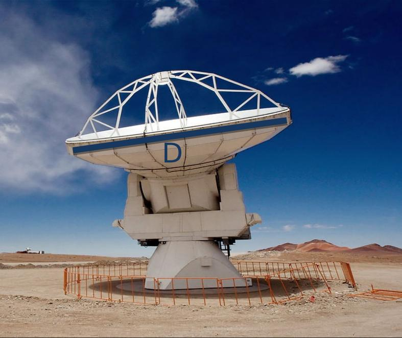
One antenna the resolution goes  $\lambda/D$ , where  $D$  is the diameter of the antenna.
