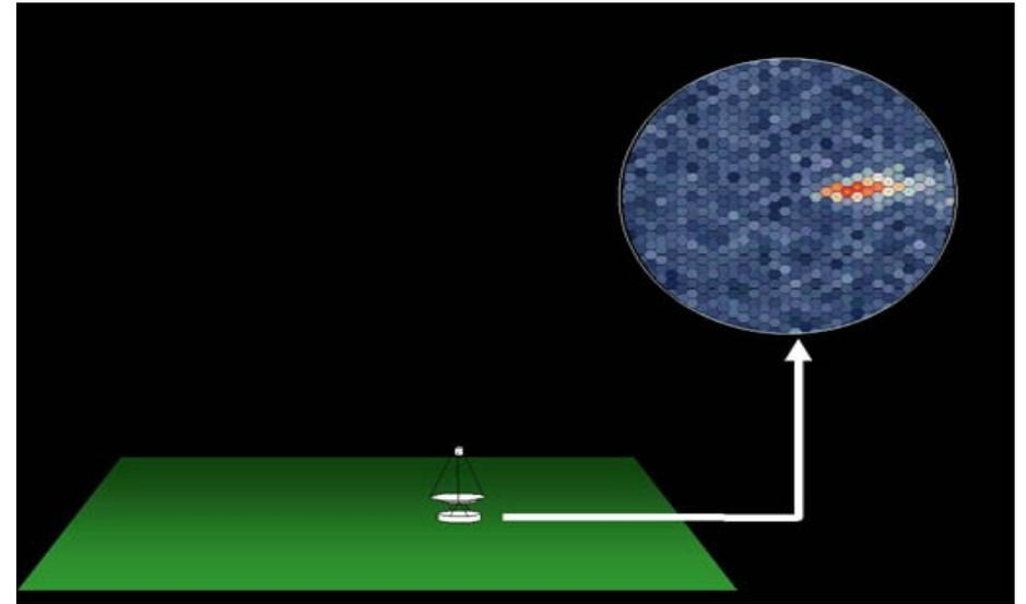
Air showers from gamma rays with  $E > 100$  GeV develop at a height of about 10 km. A pool of Cherenkov light from the shower with a radius of ~120 m reaches the ground.
