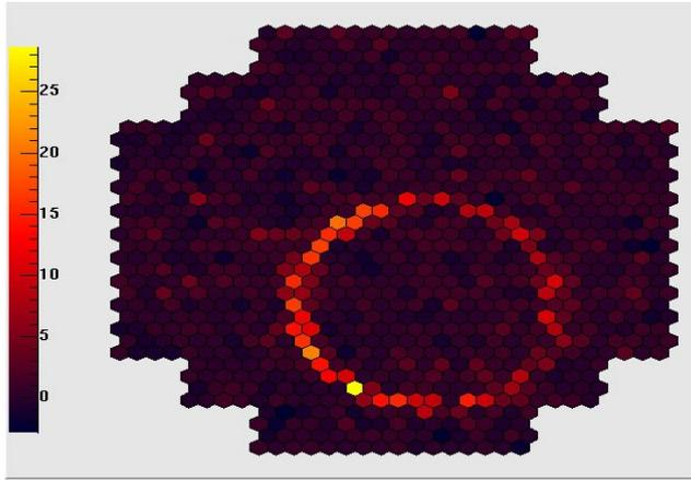
Muons that hit the telescope leave a ring-shaped Cherenkov light signal and are easily identifiable. Muons that pass the telescope at some (not too large) distance can leave a signature that is not easy to distinguish from the image of an air shower. Due to the large muon flux in the atmosphere, this is a considerable source of background.
