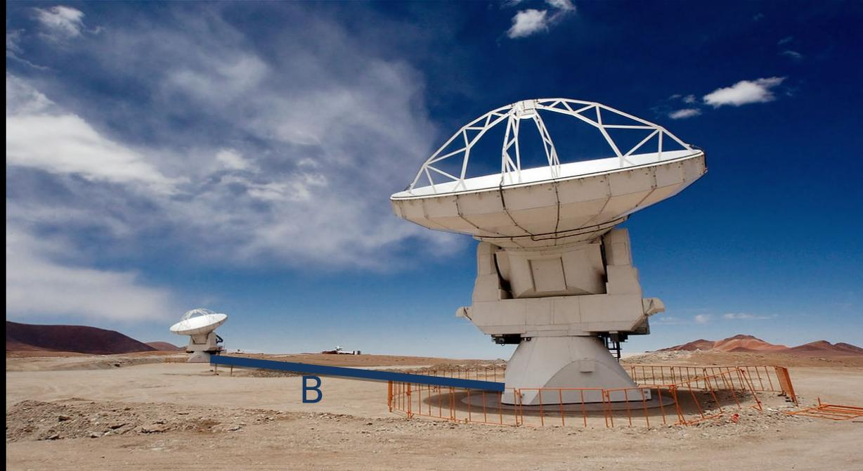
Two antennas the resolution goes  $\lambda/B$ , where  $B$  is the baseline between the two antennas.
