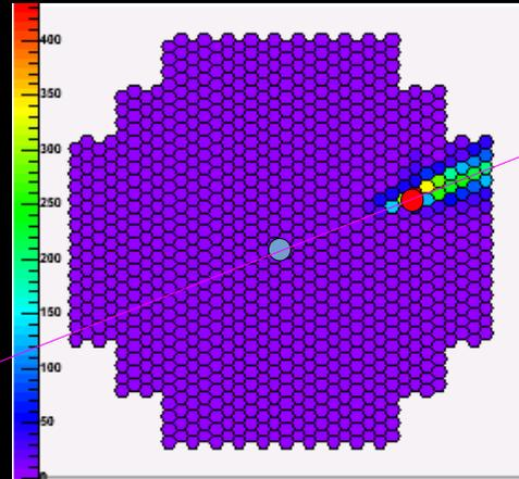
Geometrical determination of the shower impact point on the ground provides a better understanding of the shower geometry.
