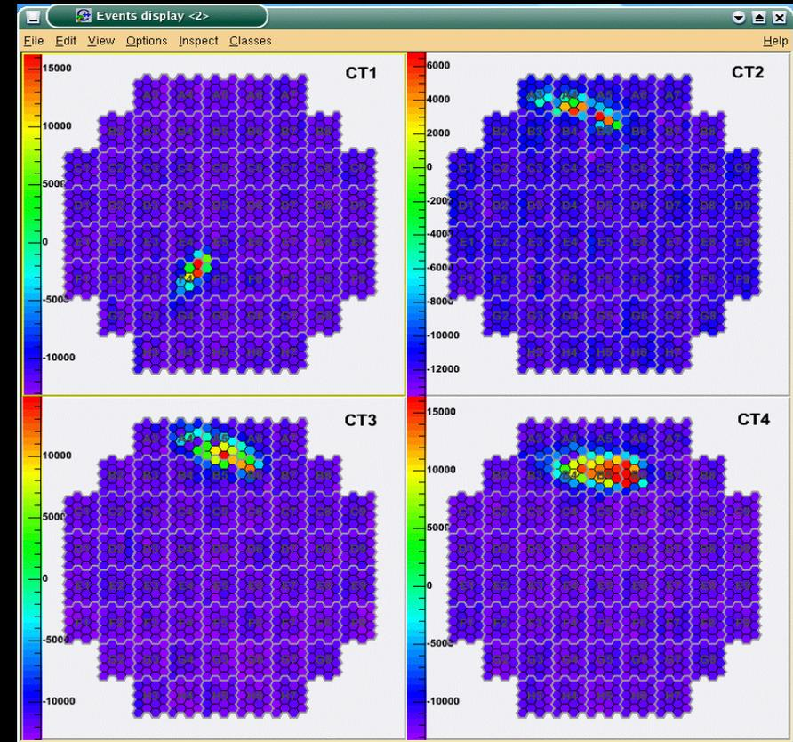
With several telescopes, a stereoscopic (or multiscope) view of a single shower is possible. This allows to reconstruct the shower geometry and to reject background signals.
