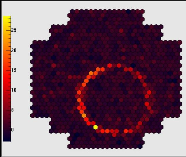
Muons that hit the telescope leave a ring-shaped Cherenkov light signal and are easily identifiable.
