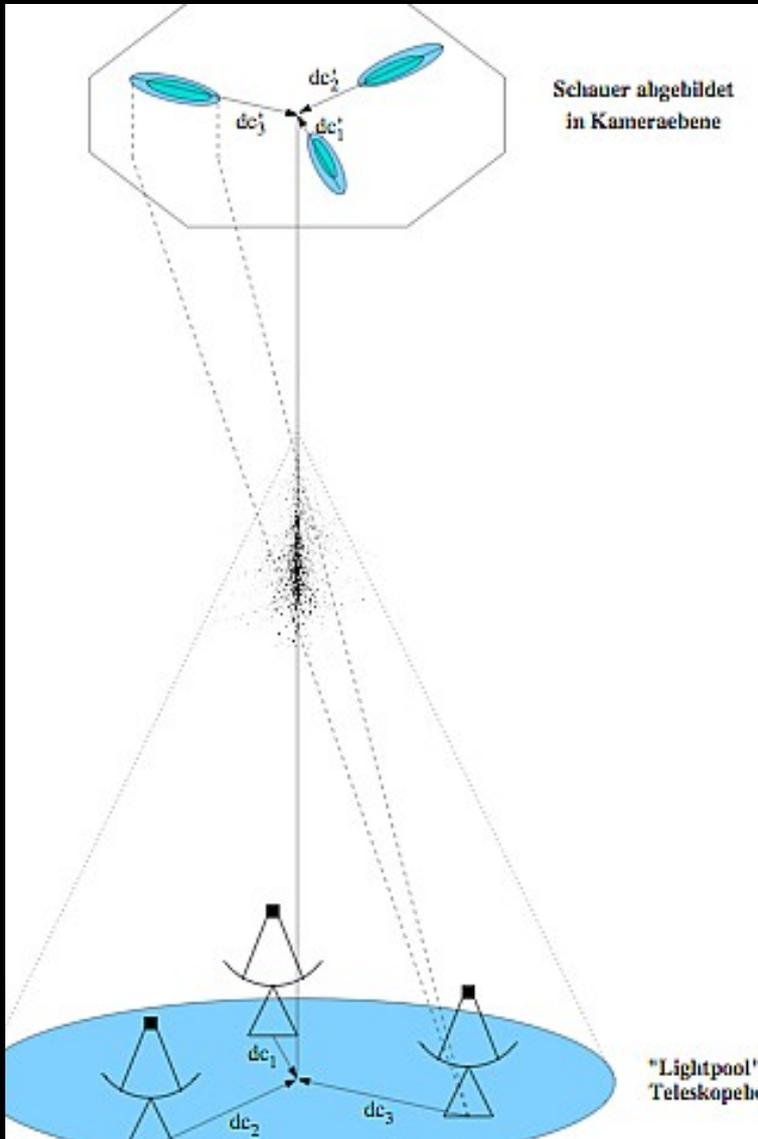
The image of the air shower that is projected onto the camera has the form of an ellipse.
