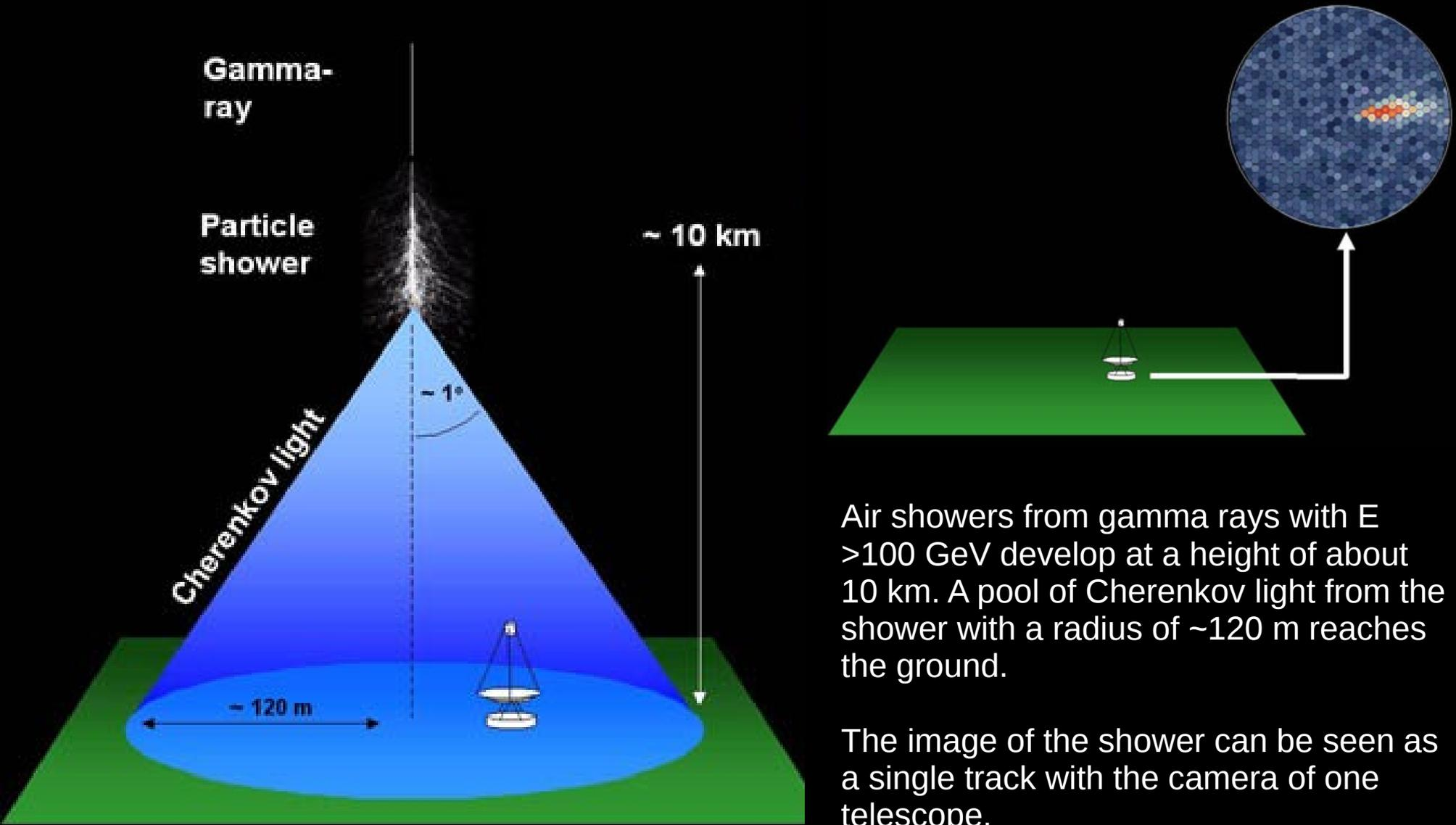
Air showers from gamma rays with  $E > 100$  GeV develop at a height of about 10 km. A pool of Cherenkov light from the shower with a radius of  $\sim 120$  m reaches the ground.
