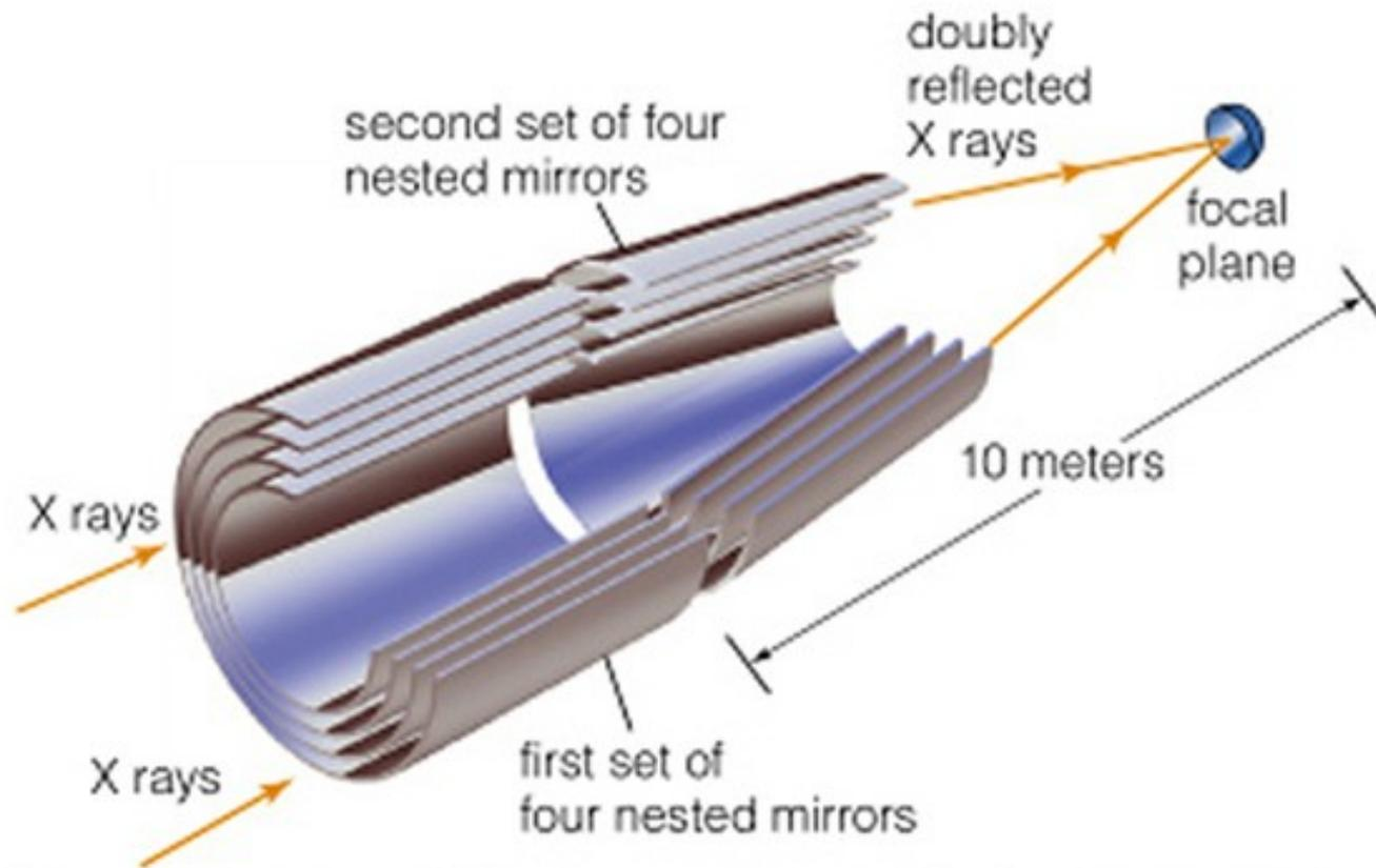
Mirror elements are 0.8 m long and from 0.6 m to 1.2 m in diameter.
